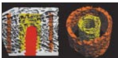
Fig 2 Three-dimensional segmented microCT images. The implant is marked in red, whereas bone is shown in grey. The 2 trabecular volumes of interest are shown in orange (outer ring, “nonaffected bone”) and yellow (inner ring).
