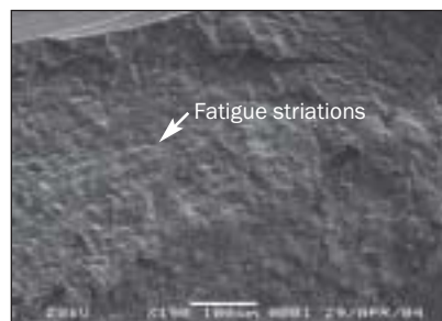
Fig 6d SEM of boxed area in Fig 6c at higher magnification showing fatigue striations. Sample 3i/4/0.
