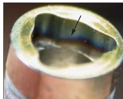
Fig 7c Blue discoloration (arrow) within the internal connection of the Replace Select implant.
