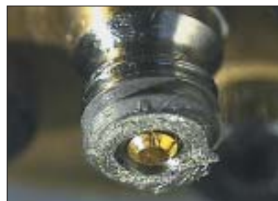
Fig 6a Fracture of implant at the third to fourth thread region. Gold-Tite screw not involved. Sample 3i/4/0.
