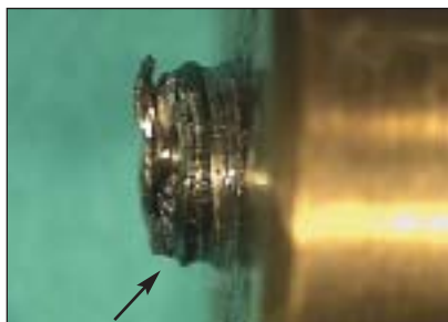
Fig 4a Implant fracture at the first thread (arrow). Sample BR/4/0.
