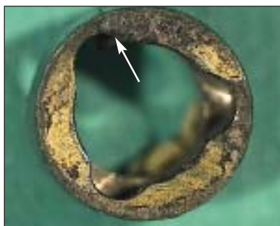
Fig 7a Crack at thinnest section of internal configuration. Sample RS/3/0.
