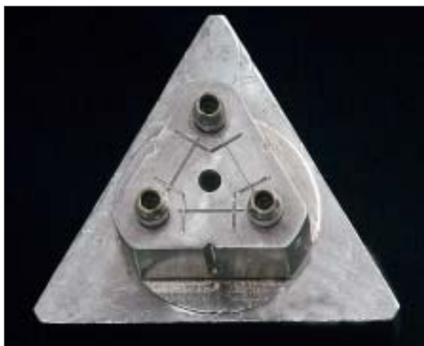
Fig 1 Master metal model with implant replicas (10 mm apart).
